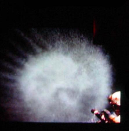
150 gpm at 100 psi (567.81 lpm at 6.89 bar)
